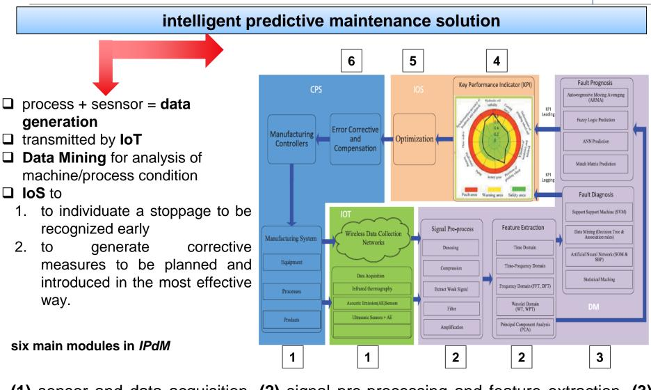
(1) sensor and data acquisition, (2) signal pre-processing and feature extraction, (3) maintenance decision-making, (4) key performance indicators, (5) maintenance scheduling optimization, (6) feedback control and compensation.
