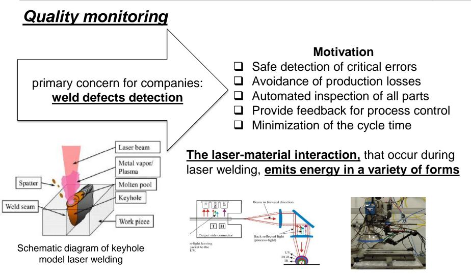
different on-line inspection systems have being developed
