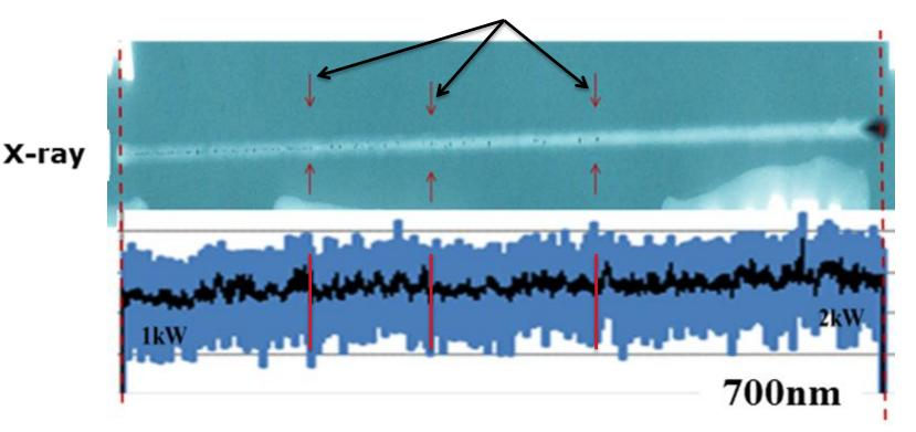
laser power ramped up from 1 to 2kW as welding proceeded, to increase the level of penetration and correspondingly decrease the internal porosity content
